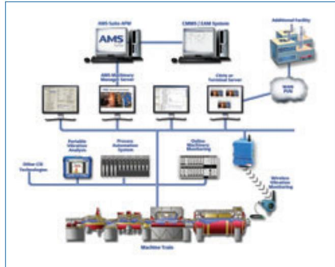
*A wide area network allows communication and analysis of machinery health information around the globe.*
