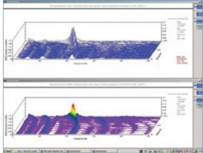
Viewing a waterfall plot in color allows you to see the difference in the amplitudes more readily.
