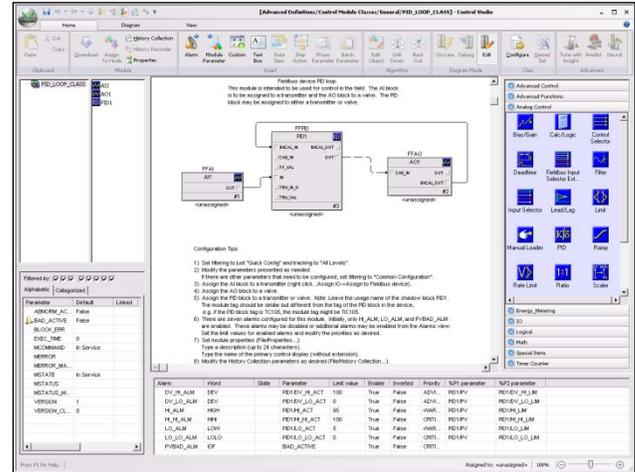
PID loop function block diagram
