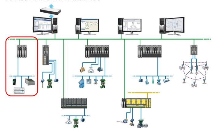
EIOC integrated into the DeltaV system (simplex EIOC shown)
