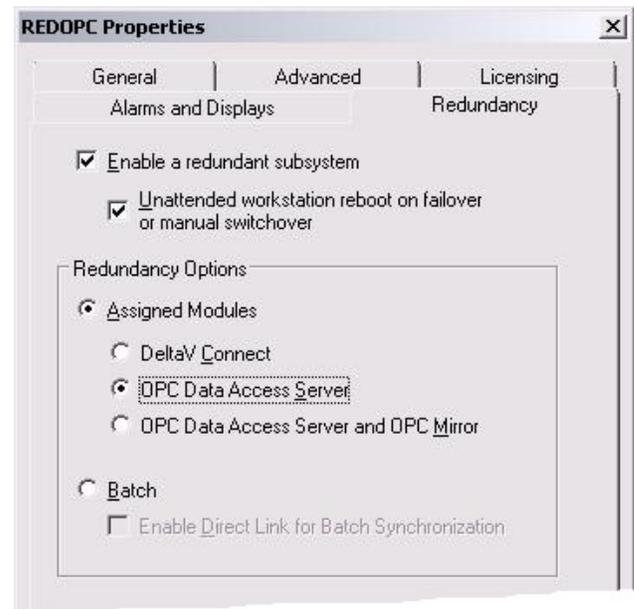
Although there are two physical Application Stations that host the redundant OPC servers, they are seen by the DeltaV system as a single workstation. The Application Station pair is known by the name configured for the initial active OPC server node (e.g. **REDOPC**). The initial standby OPC server node has the same name appended with **\_S** (e.g. **REDOPC\_S**). The Application Station pair appears in the DeltaV Explorer system tree as a single icon.
