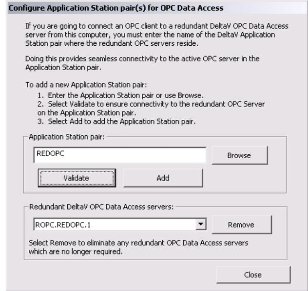
Redundant OPC servers are supported only on the Application Station. Only the redundant OPC servers, Assigned Modules subsystem and DeltaV and/or 3<sup>rd</sup> party OPC applications associated with the OPC redundancy solution shall be installed and run on the Application Station pair. Other DeltaV subsystems may not be enabled on the Application Station pair. Other non-OPC related DeltaV applications are not supported for use on the Application Station pair.
