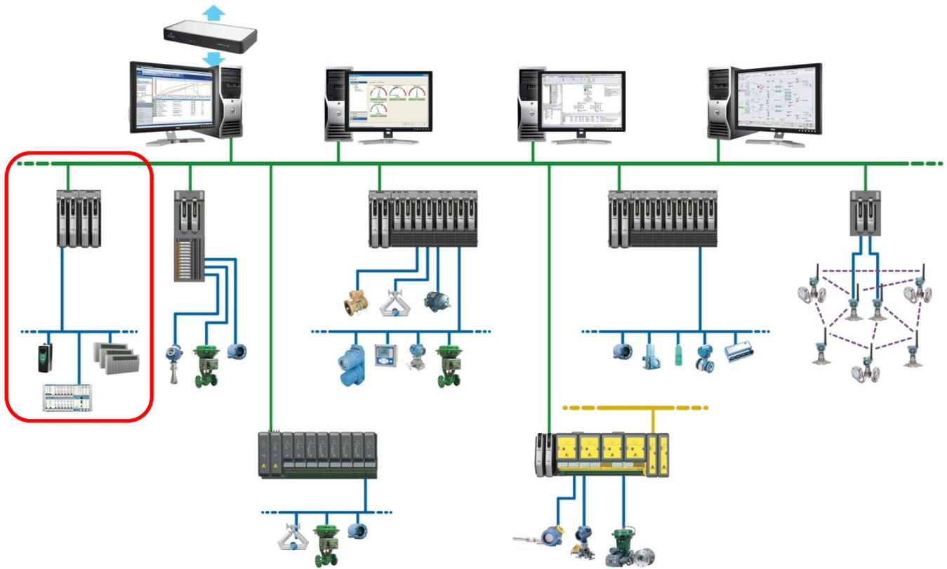
*The DeltaV system with S-Series VIM and Ethernet I/O integration (simplex VIM and DeltaV controller shown)*
