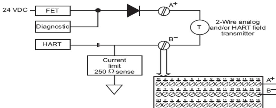
Wiring diagram and terminations for HART analog input channels
