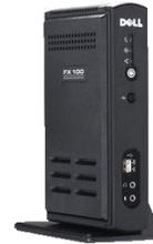
The FX100 has dual video outputs and will support DeltaV Dual Monitor workstations
