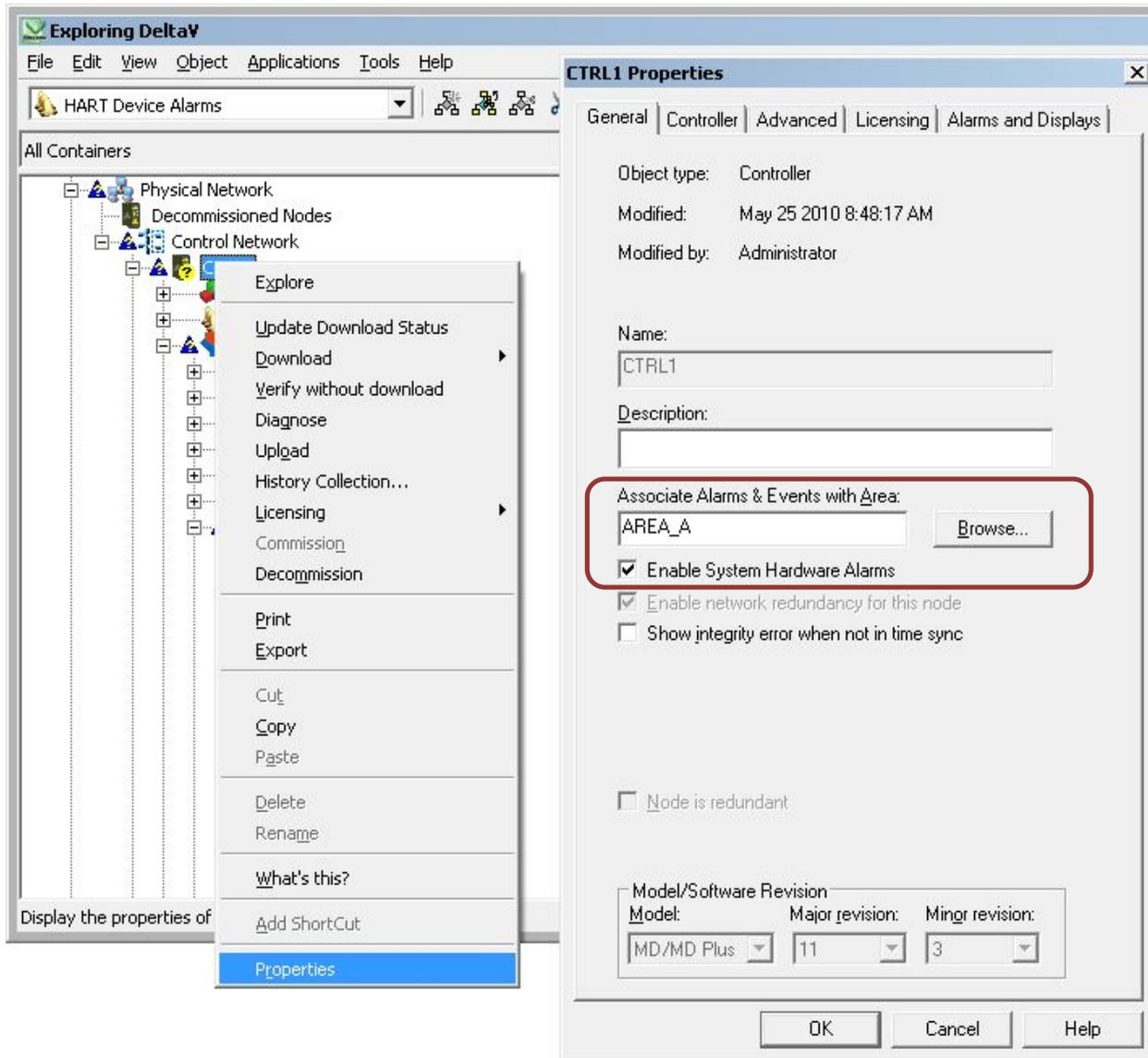
Figure 2 Controller Alarm and Events Area Association for Integrity Reporting
