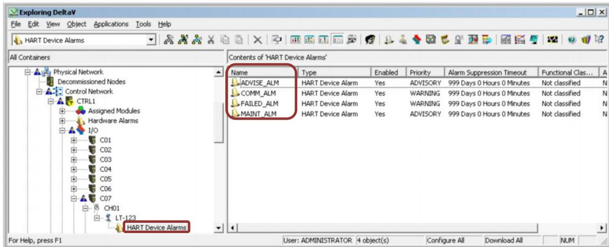
Figure 1 HART Device Alarms
