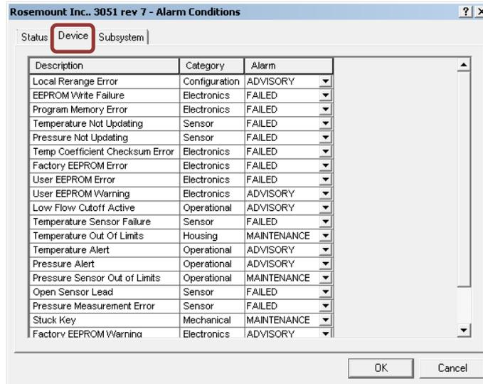
Figure 10 Configuring Alarm Conditions—Device
