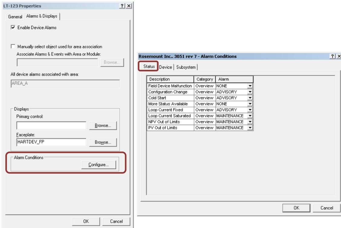
Figure 9 Configuring Alarm Conditions—Status
