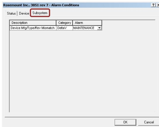
Figure 11 Configuring Alarm Conditions—Subsystem
