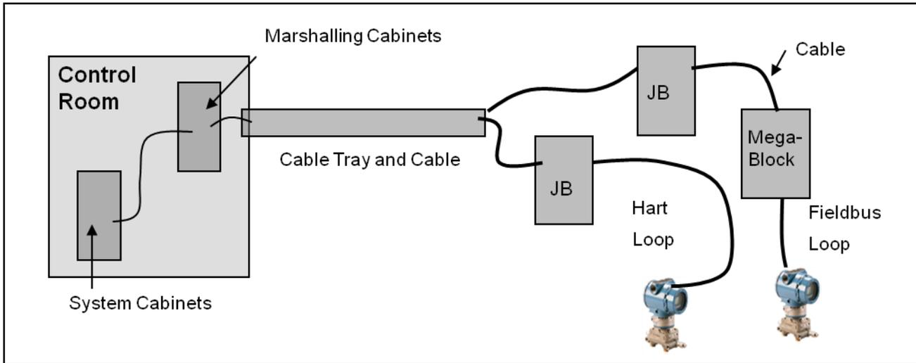
Figure 2 – Typical Cable Routing
