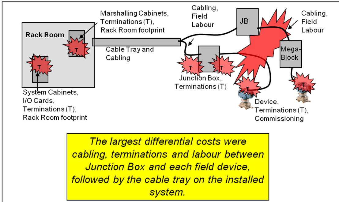
Figure 4 – Largest Differential Cost Locations – Installed System
