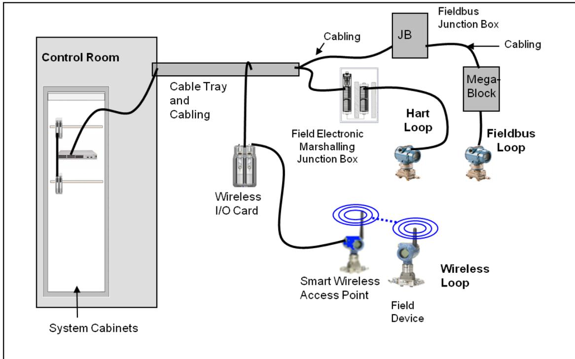
Figure 5 – Example of I/O on Demand Installation
