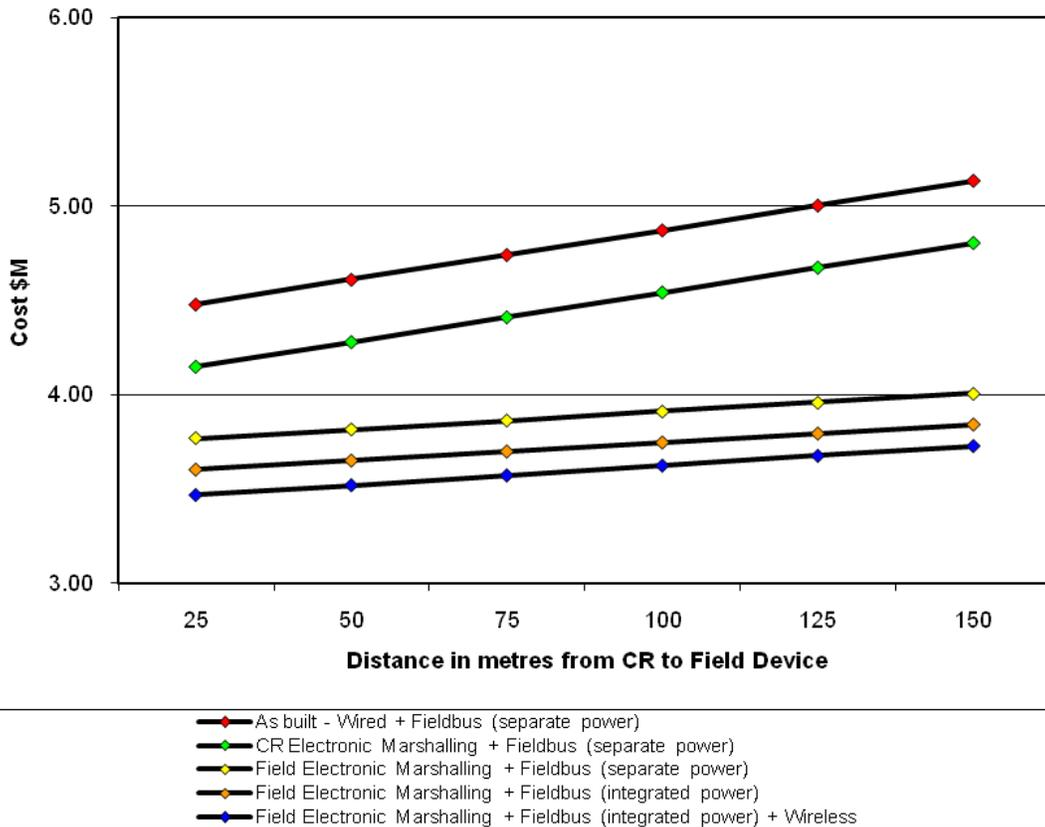
Figure 3 – Analysis of Cost over Distance on Platform PAS
