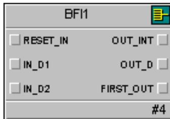
Figure 9: Boolean Fan Input Function Block
