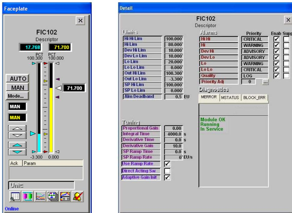
Figure 5. DeltaV Connect™ Solution for Moore® Systems Single Loop PID Faceplate and Detail Displays
