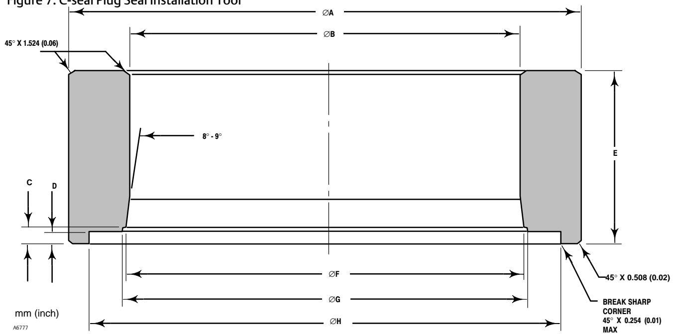
Figure 7. C-seal Plug Seal Installation Tool
