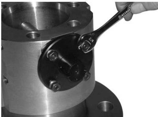
Figure 7. Bolt Up the Packing Flange
