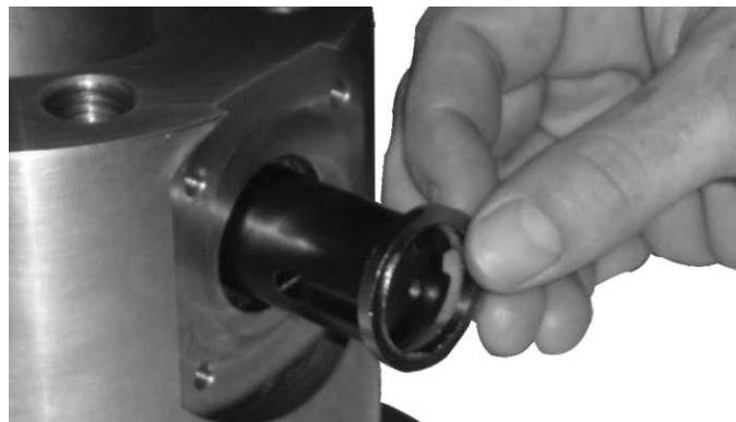
Figure 5. Insert Top End Ring
