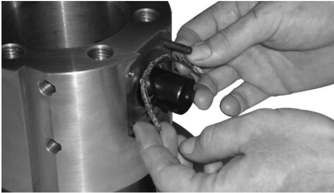
Figure 6. Use Packing Flange
