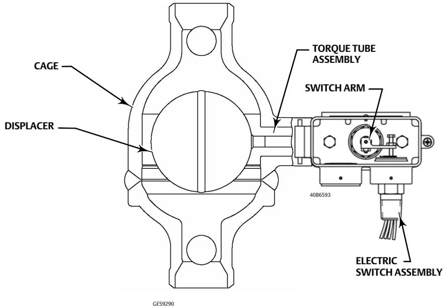
Figure 3 shows a sectional view of the 2100 switch positioned for low level activation. The nozzle, flapper, and magnet are on the opposite side of the torque tube, so that downward displacer travel moves the flapper away from the nozzle.
