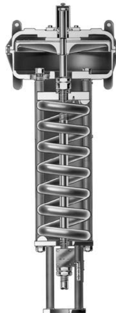
Figure 1. Sectional view of Fisher 657 Size 100 Actuator
