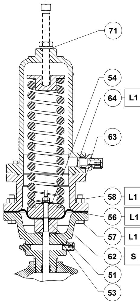
NOTE: KEYS 64 AND 71 ARE USED ONLY FOR PRESSURE-LOADED ACTUATORS.
