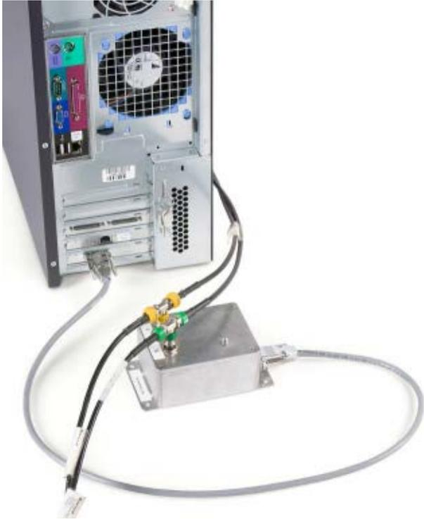
*Figure 1. Application Station with LCN interface card and LCN network cables*
