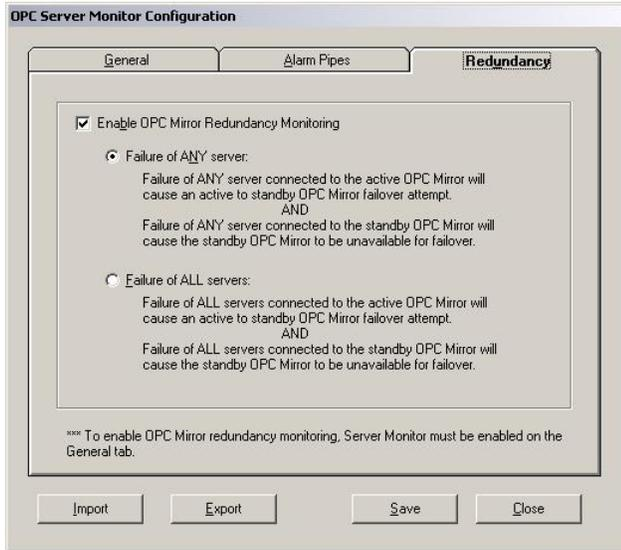
Redundant OPC Mirror is supported only on the DeltaV Application Station. Simplex OPC Mirror may be used with redundant DeltaV OPC Servers. The simplex OPC Mirror may be installed on another DeltaV workstation or a 3rd-party workstation. The simplex OPC Mirror does not provide the Server Monitor feature included in the redundant OPC Mirror.
