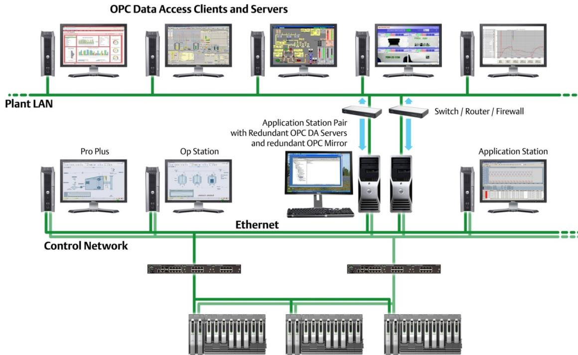
*Redundant OPC Mirror provides highly reliable OPC Server-to-server data transfer.*
