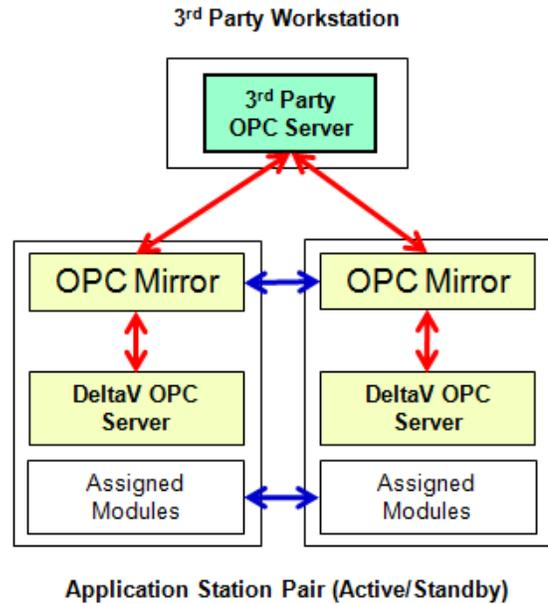
A 3<sup>rd</sup>-party OPC server may also be installed on a 3<sup>rd</sup>-party workstation. In this architecture, the active OPC Mirror and standby OPC Mirror will be configured to connect to the remote 3<sup>rd</sup>-party OPC Server.
