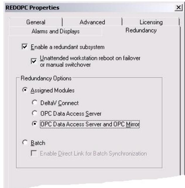
Although there are two physical Application Stations that host the redundant OPC Mirror, they are seen by the DeltaV system as a single workstation. The Application Station pair is known by the name configured for the initial active OPC Mirror node (e.g. *REDOPC*). The initial standby OPC Mirror node has the same name appended with *\_S* (e.g. *REDOPC\_S*). The Application Station pair appears in the DeltaV Explorer system tree as a single icon.
